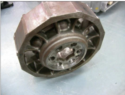
Figure 5 / The core or rotor is made of very strong rare earth metal permanent magnets
